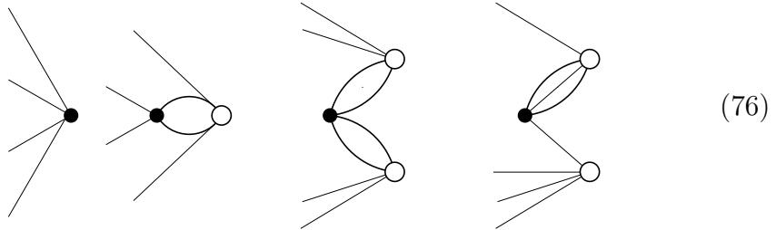
The first diagram represents simply  $| \Phi_{ij}^{ab} \rangle \langle \Phi_{ij}^{ab} | H_N | \Phi_0 \rangle = | \Phi_{ij}^{ab} \rangle \langle ij | ab \rangle$ . In the second diagram  $H_N$  and  $T_2$  are connected by two lines. The last two diagrams are quadratic in  $T_2$ . Note now that it is impossible to have a contribution containing the third power  $T_2^3$  that is connected with  $H_N$  and has four free lines.
