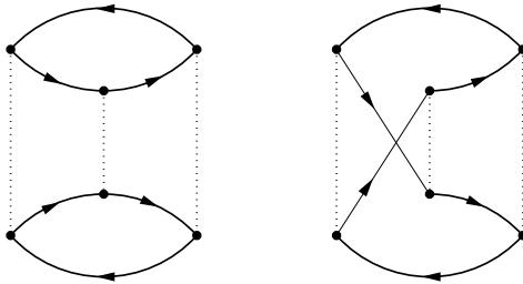
Note that the first representative contains two loops. A loop contains oriented non-dashed (= orbital) lines which, when followed starting at a certain vertex, bring us back to this vertex. The second diagram has one loop. Let the number of loops be  $l$ . Let the number of hole lines in a certain diagram be  $h$  (both diagrams have  $h = 4$ ). Then the overall sign is  $(-1)^{l+h}$ . So the first representative has sign +1 and the numerator
