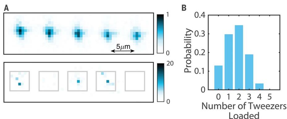
**Fig. 2. Molecule tweezer array.** (A) (Top) Image of optical tweezer array of single molecules, averaged over 500 shots. (Bottom) Single-shot image showing three occupied tweezer traps. The gray boxes represent the regions over which photon counts are summed. Color scale indicates signal per pixel. (B) Probability versus number of tweezer traps loaded. The average loading probability per trap is 34%.
