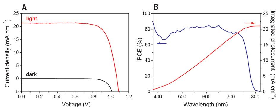
**Fig. 1. Performance of perovskite solar cell.** (A) Current density–potential curve ( $J$ – $V$ ) of the perovskite solar cell under dark and simulated AM 1.5G  $100 \text{ mW cm}^{-2}$  illumination. (B) IPCE spectrum of the perovskite solar cell and the integrated photocurrent with the AM 1.5G solar spectrum.
