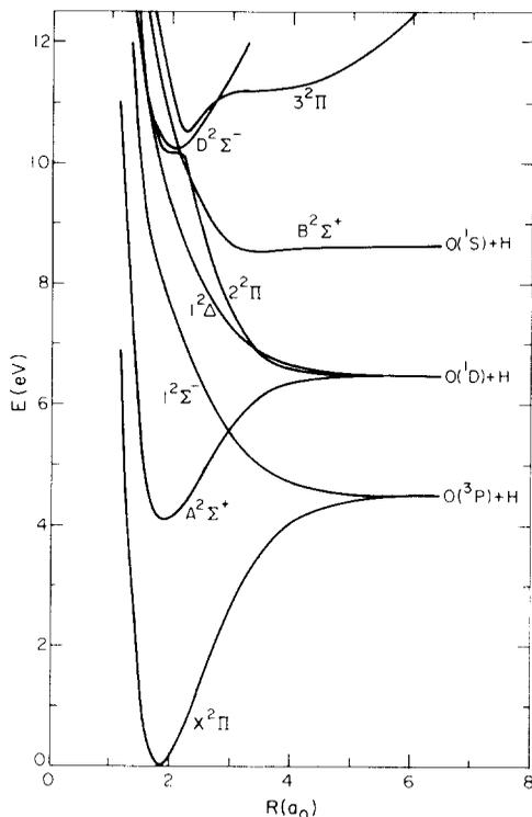
FIG. 1. Calculated potential energy curves of the doublet states of OH.
