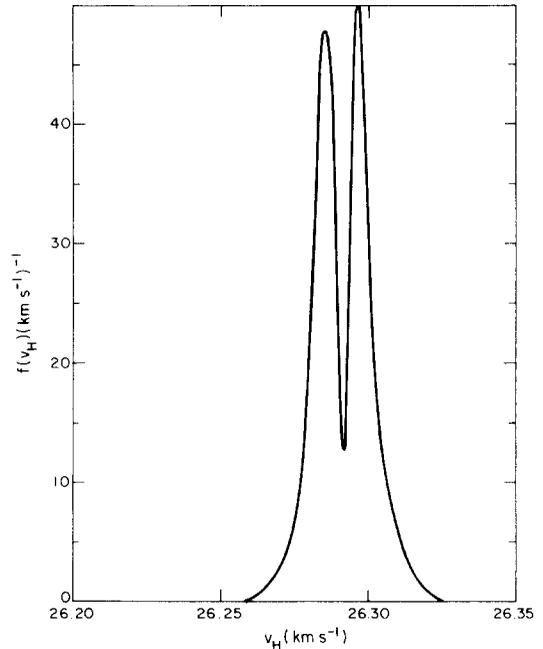
FIG. 5. The hydrogen atom velocity distribution resulting from the photodissociation of OH by absorption of Lyman  $\alpha$  radiation into the  $1^2\Delta$  or  $2^2\Pi-3^2\Pi$  states.
