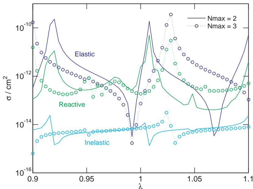
FIG. S1: Elastic, inelastic, and reactive NH + NH collision cross sections for different basis sets as a function of the scaling parameter  $\lambda$ , calculated at a collision energy of  $10^{-6}$  K and a magnetic field strength of 1 G.
