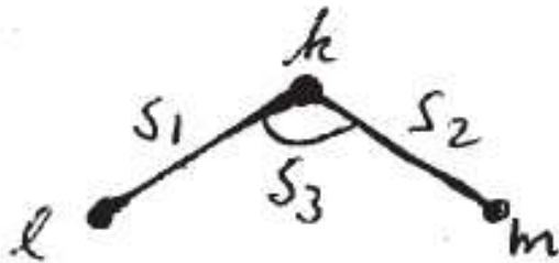
Figure 6: Example: Internal coordinates of water molecule ( s_1 = \Delta r_{kl} , s_2 = \Delta r_{km} , s_3 = \Delta \Theta_{klm} ).
